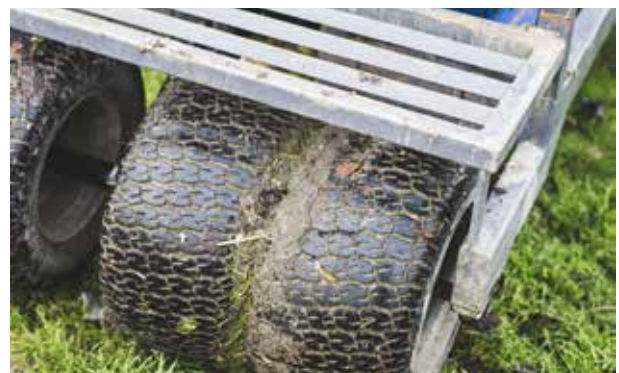
Rollers put turf back in position
